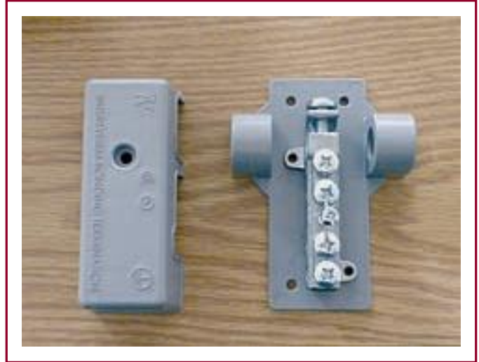
EXHIBIT 250.37 A listed intersystem bonding termination providing the required number of terminals (minimum of three) for connecting other building systems to the grounding system of the electrical power supply.
